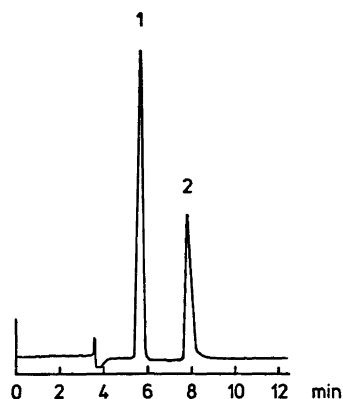
Fig. 1. Isocratic separation of the isomers menthone (1) and isomenthone (2) on \mu -Porasil. Flow rate 1 ml/min. Temp. ambient.
